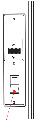
On/Off switch for interior ceiling lighting
